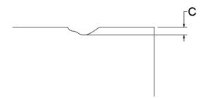
Modules that have cracks/chips which extend into areas above the copper electrodes must be rejected regardless of dimension:
