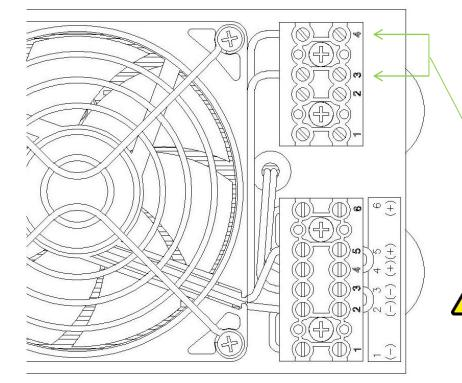
The external fan speed can be optionally controlled using pulse width modulation at a recommended 5 kHz to 25 kHz frequency applied at terminal position 4 (SPD CTRL, brown wire). The TC-720 temperature controller can be used to provide this PWM signal to reduce the audible noise at low cooling demands (use 5400Hz frequency setting). Electrical ground to terminal position 4 will reduce fan speed.
