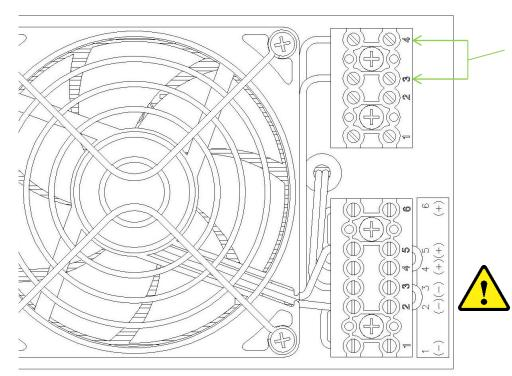
The external fan speed can be optionally controlled using pulse width modulation at a recommended 5 kHz to 25 kHz frequency applied at terminal position 4 (SPD CTRL, brown wire). The TC-720 temperature controller can be used to provide this PWM signal to reduce the audible noise at low cooling demands (use 5400Hz frequency setting). Electrical ground to terminal position 4 will reduce fan speed.
