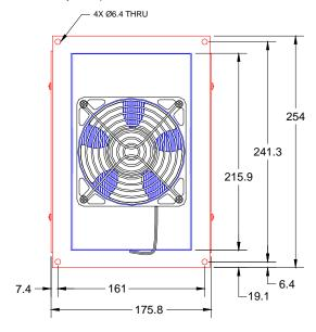
NOTE: 1. ALL DIMENSIONS IN MILLIMETERS 2. COLD SIDE SHOWN IN BLUE; HOT SIDE SHOWN IN RED
