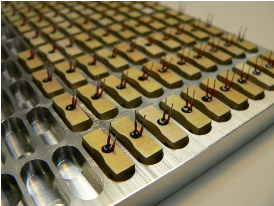
Thermistors epoxied into aluminum cold plates
