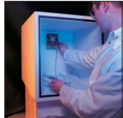
Engineer tests the thermal performance of a prototype refrigerator for the food service industry.
