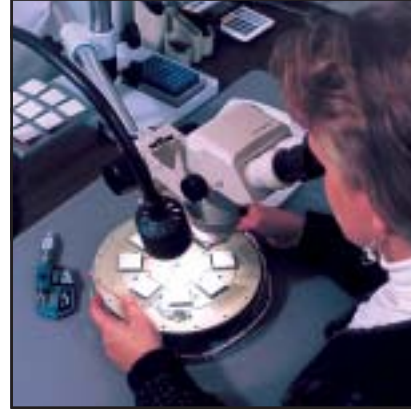
Assembler inspects solder joints on an air cooler.
