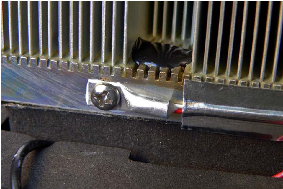
Sensor monitoring the base plate temperature of a finned heat sink
