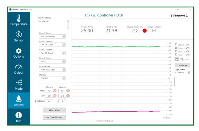
The ALARMS menu provides settings for how the controller will respond if an alarm condition occurs. It also provides settings for fan-speed control.
