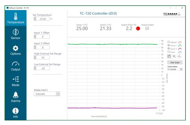
The allowable SET TEMPERATURE is limited to the range defined by the HIGH EXTERNAL SET RANGE and the LOW EXTERNAL SET RANGE. Using an appropriate set range helps to prevent inadvertently using a set temperature that would be inappropriate for the TE device.
