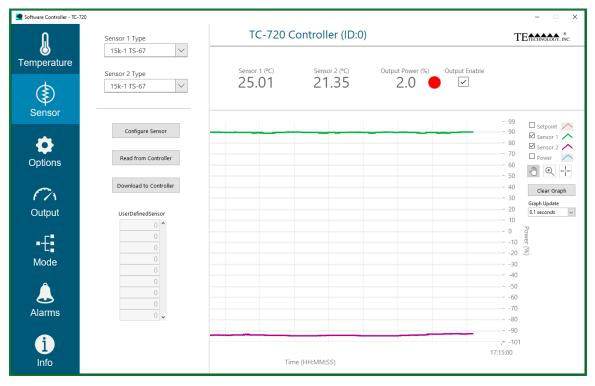
Most of the sensor options correspond to various negative-temperature-coefficient thermistors that TE Technology offers. The temperature-resistance tables for the various sensors are provided in the appendix for reference. Additional information on the thermistors is available online at <u>www.tetech.com</u>.
