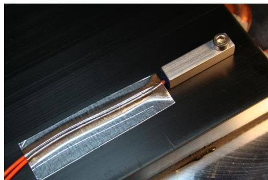
NOTE: When possible, it is recommended that at least 50 mm of the thermistor's wire be thermally connected to the cold side of the TE device. This can be accomplished by placing aluminum tape over the thermistor wires and adhering the wires and tape to the cold side of the cooler. If this is not done, the thermistor wires will be at a different temperature than the cold side and they will add or remove heat in the
