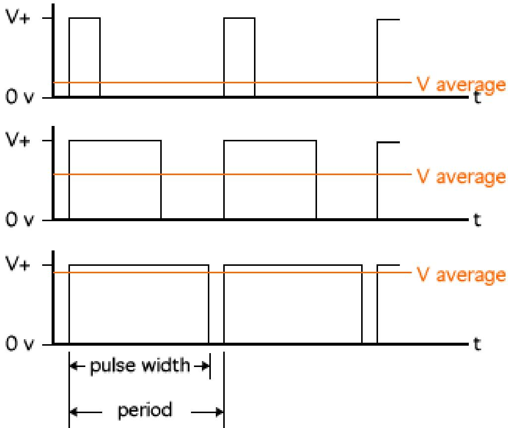
The important advantage to PWM is that it does not cause the extreme temperature excursions that are experienced with a thermostatic control system. This helps to extend the life and reliability of the TE devices. An added benefit is that the controller does not generate a large amount of waste heat, so a large heat sink is not usually required.
