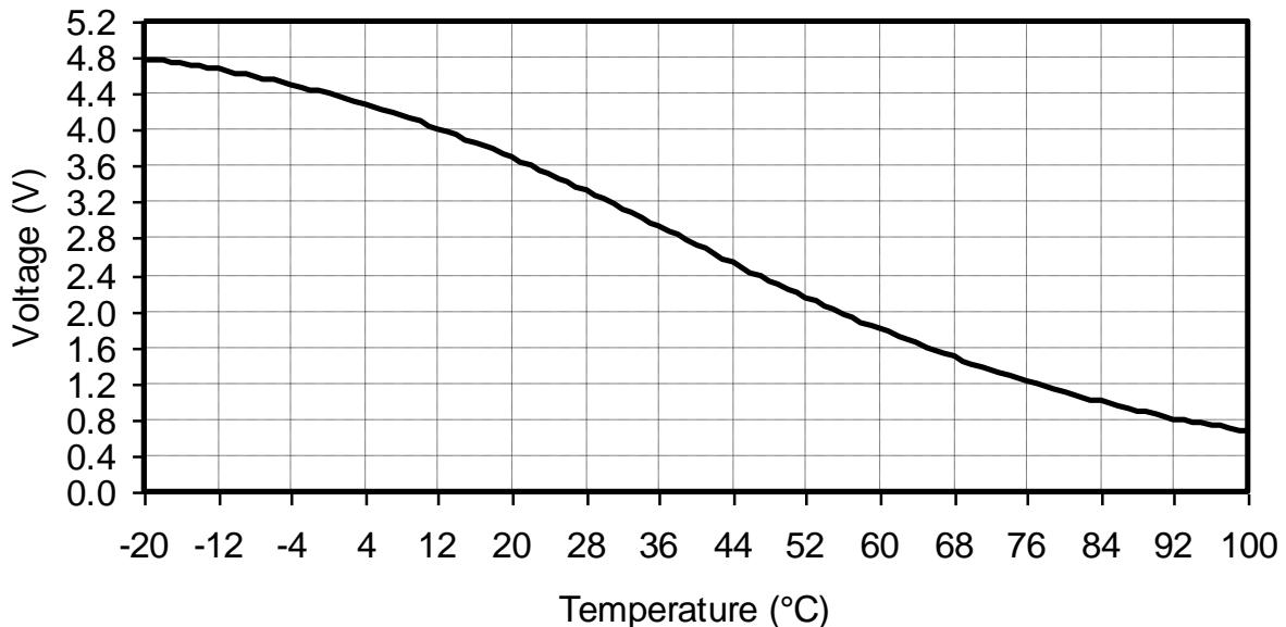
**Potentiometer Voltage Vs. Set-point Temperature**
