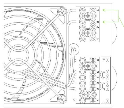
The external fan speed can be optionally controlled using pulse width modulation at a recommended 5 kHz to 25 kHz frequency applied at terminal position 4 (SPD CTRL, brown wire). The TC-720 temperature controller can be used to provide this PWM signal to reduce the audible noise at low cooling demands (use 5400Hz frequency setting). Electrical ground to terminal position 4 will reduce fan speed.
