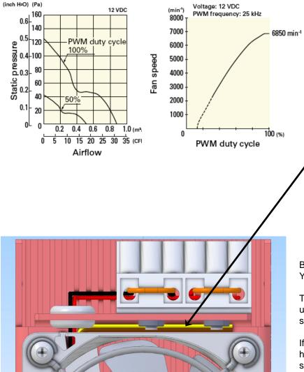
The fan speed operates at 100% as shipped. DO NOT OPERATE THE CP-035HT IN COOLING MODE WITH A PWM DUTY CYCLE OF LESS THAN 50%. DO NOT ALLOW HEAT SINK OR COLD PLATE TEMPERATURES TO EXCEED 100  $^{\circ}$ C.
