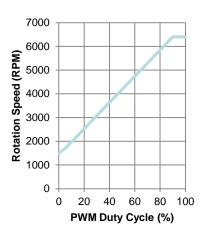
The external fan speed can be controlled using pulse width modulation at a recommended 5KHz to 25 kHz frequency applied at terminal position 4 (SPD CTRL, brown wire). The TC-720 temperature controller can be used to provide this PWM signal to reduce the audible noise at low cooling demands (use 5400Hz frequency setting). Electrical ground to terminal position 4 will reduce fan speed.
