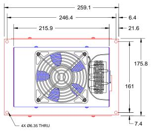
NOTE: 1. ALL DIMENSIONS IN MILLIMETERS 2. COLD SIDE SHOWN IN BLUE; HOT SIDE SHOWN IN RED
