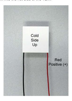
If the TEM has one substrate that is wider than another, as with some micro TEMs, the answer is again simple because the hot side of the TEM is the larger of the two sides. Once you know which side is the hot side all thermoelectric TEMs follow the same wire convention: the positive wire is always on the right side wire when the hot side of the TEM is placed down on a table and both wires are pointing towards you.
